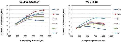
Fig. 4- Slide OUT ejection shear stress for specimens pressed by CC and WDC-60°C (12.7 mm, 5 SPM).
