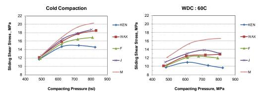
Fig. 7- Ejection performance (Sliding AVG) for Mixes F, J and M obtained by CC and WDC- 60°C (12.7 mm, 5 SPM).
