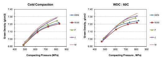
Fig. 6- Compressibility curves obtained for Mixes F, J and M obtained by CC and WDC- 60°C (12.7 mm, 5 SPM).
