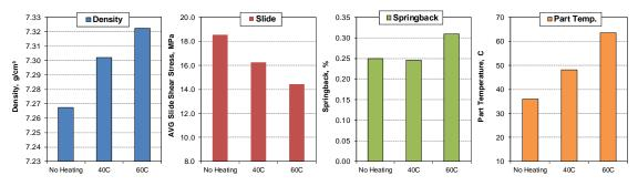
Fig. 12- Effect of die temperature on density, ejection slide shear stress and springback (12.7 mm, 5SPM)
