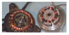
Figure 7. Conventional brush DC motor with a lap winding and the SMC stator of a brushless DC motor with a concentrated winding.
