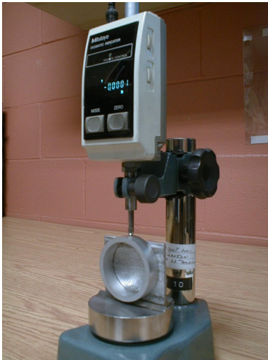
Figure 1. Fixture used to measure the outside diameters of green and sintered rings.
