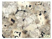
combined carbon: 0.15% tempered at 200°C/60 min/N $_2$
