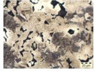
combined carbon: 0.55% tempered at 200°C/60 min/N $_2$
