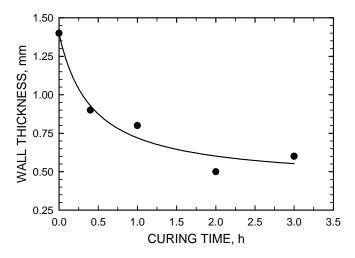
Figure 11. Effect of curing time on the minimum wall thickness required to drill 3.18 mm diameter holes in the gear teeth for part density of 6.8 g/cm<sup>3</sup> (Feed rate: 0.2 mm/rev, Speed: 3420 rpm).
