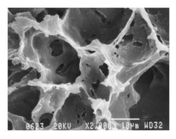
Figure 7. Illustration of the thin network of lubricant throughout cured TRS specimens pressed from the BM system.
