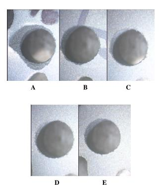
Figure 10. Break-out at the exit of 6.35 mm diameter holes drilled at a feed rate of 0.2 mm/rev and a cutting speed of 3420 rpm for material cured at 175°C for A) 0 h, B) 0.5 h, C) 1.0 h, D) 2.0 h and E) 3.0 h.
