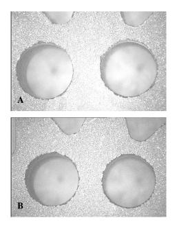
Figure 12. Break-out at the exit of 6.35 mm diameter holes drilled at a feed rate of 0.2 mm/rev and a cutting speed of 3420 rpm cured at 230°C for A) 0.5 h and B) 1.0 h.
