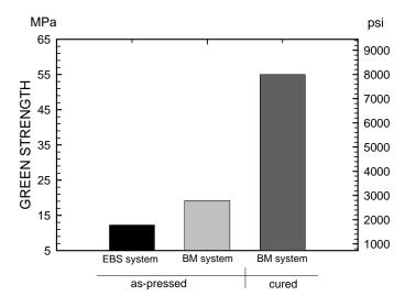
Figure 6. Effect of the curing treatment on green strength of 0.64 cm thick specimens pressed from the BM system and comparison with the EBS system.
