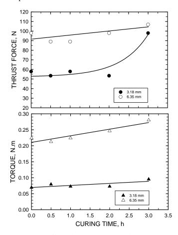
Figure 9. Effect of curing time at 175°C on a) Thrust force and b) Torque required to drill holes in material containing the new BM lubricant system (Speed: 3420 rpm).
