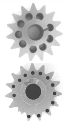
Figure 2. Location of a) 6.34 mm and b) 3.18 mm diameter holes drilled for machinability evaluation.
