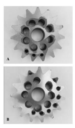
Figure 8. Break-out zones at the exit of the tools when drilling in materials containing A) EBS and B) the BM system as lubricant.
