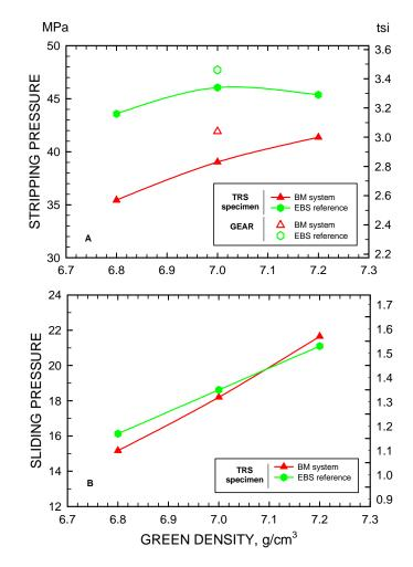
Figure 4. Stripping and sliding pressures required to eject TRS and gears made from BM and EBS lubricating systems.
