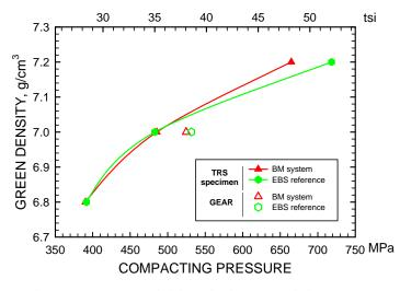
Figure 3. Compressibility of mixes containing BM and EBS lubricating systems on lab and production presses.
