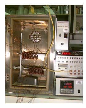
Figure 1: Thermal chamber assembly with the temperature programmer and recorder.
